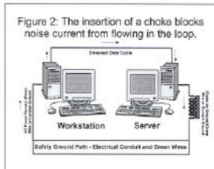
A choke is nothing more than a coil of wire wound around a core of iron or steel. As the loop current flows through the device the magnetic field from this current induces a current that is opposite in polarity from the original current. The result is that the two currents want to cancel one
